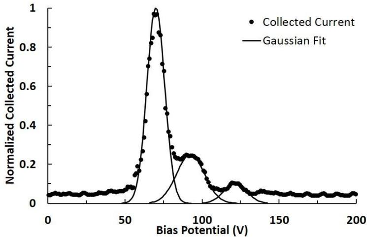
**Figure 6.** Normalized ExB probe current scan showing MaSMi's ion species mix during operation at nominal conditions in the high-temperature diffuse mode with Gaussian fits to each charge species.
