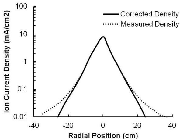
**Figure 5. Ion current density as a function of Faraday probe lateral position from thruster centerline for MaSMi operating at nominal conditions in the high-temperature diffuse mode. Traces for the unaltered measurement data and the data corrected for background charge-exchange collisions are shown.**
