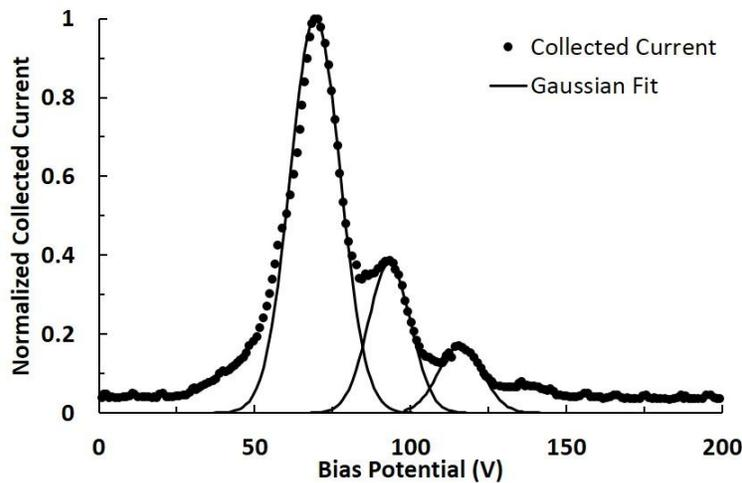
**Figure 3. Normalized ExB probe current scan showing MaSMi's beam composition during operation at nominal conditions in the low-temperature jet mode. Gaussian fits are used to identify each ion species**
