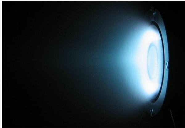
**Figure 1. MaSMi's plasma discharge while operating at 275 V and 1.2 A in the low-temperature jet mode.**
