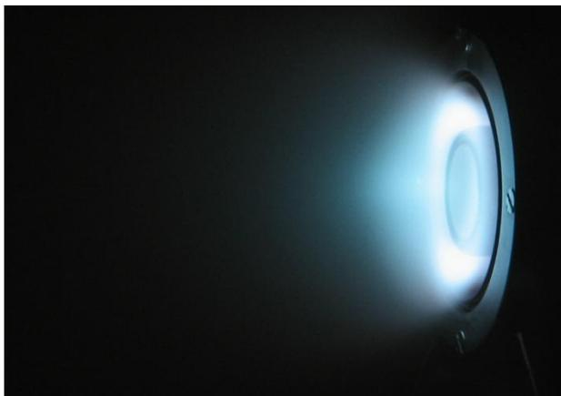
**Figure 4. MaSMi's plasma discharge while operating at 275 V and 1.2 A in the high-temperature diffuse mode.**
