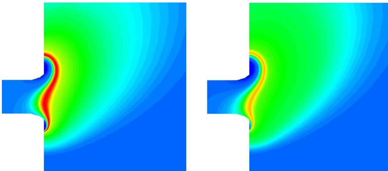
**Figure 9. Normalized electron temperature profiles for MaSMi's measured jet mode field topology (left) and assumed diffuse mode field topology (right) created by saturation of the inner magnetic circuit at elevated operating temperatures.**
