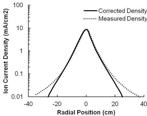
**Figure 2. Ion current density as a function of Faraday probe lateral position from thruster centerline for MaSMi operating at nominal conditions in the low-temperature jet mode. Traces for the unaltered measurement data and the data corrected for background charge-exchange collisions are shown.**
