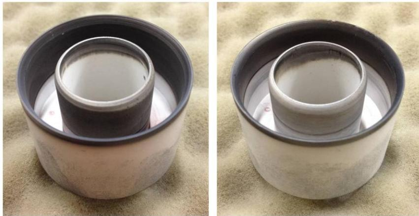
**Figure 7.** Comparison of MaSMi's discharge channel after operation in the jet mode (left) and the diffuse mode (right), showing a significant reduction in carbon deposition along the inner channel wall.
