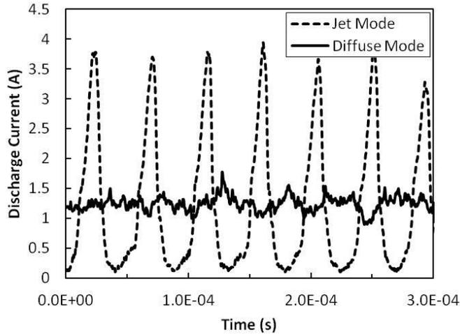
**Figure 8. Comparison of the discharge current oscillations measured during operation of the MaSMi Hall thruster in the low-temperature jet mode and the high-temperature diffuse mode.**
